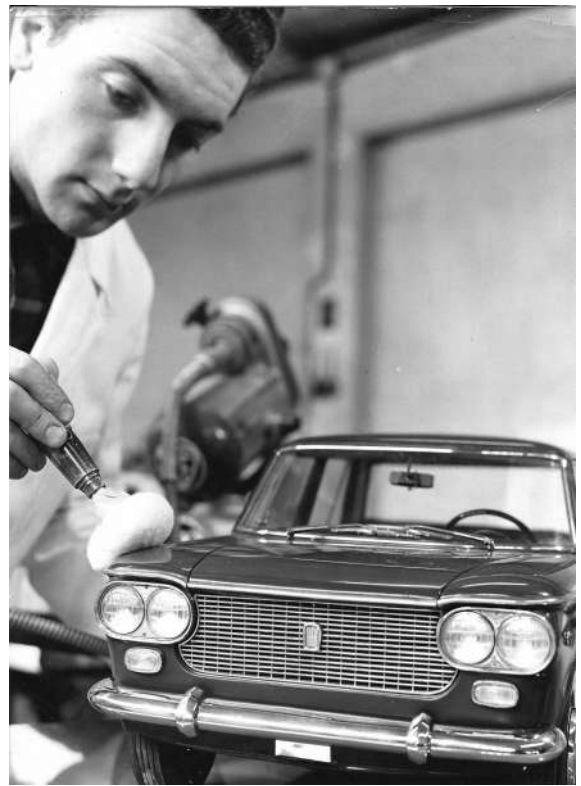
Final polishing work on the painting of the 1300/1500 saloon model in the Acerbi workshop. The imposing size and the fine detail of the model can be easily understood
