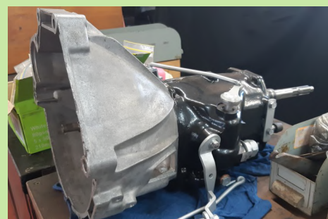
The reconditioned gearbox, sans overdrive
